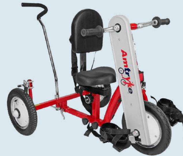
12 inch front wheel with a flat-proof insert
