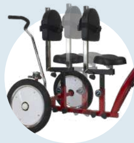
Seating can be positioned forward or back along the frame
